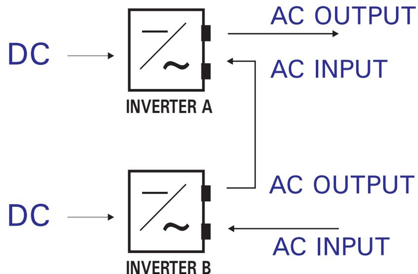
**Dual Inverter Backup Systems** - AC Output will be available as long as Inverter A or Inverter B is operational.
